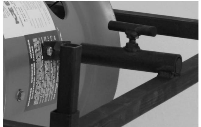
Insert bolt and place washer with lock nut on the inside and tighten.
